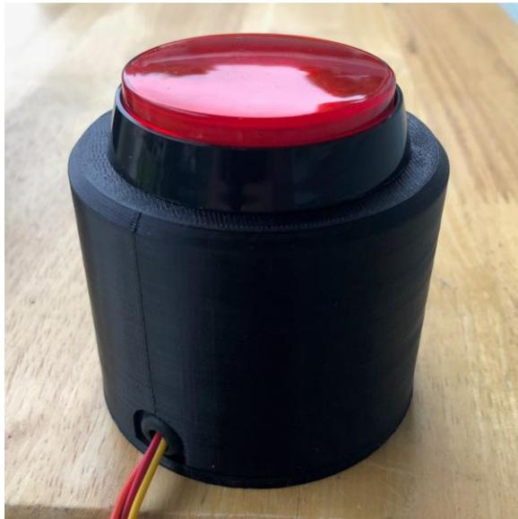
Note you will likely need to also print the nut tool in order to screw the nut on. The hardware in the kit allows you to attach the lid to the main enclosure body. The grommet protects the wires from abrasion – you will have to cut the grommet in order to put it around the cable.
