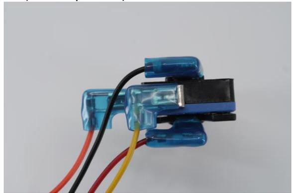
3. Place the LED into the LED holder, and make a note of which leg the flat side/cathode of the LED is contacting. You'll need to know this later when connecting the button to your project.
