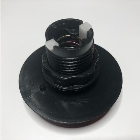
5. Insert the switch & LED assembly into the button. Note that there's an L-channel on two sides of the switch/LED assembly, line those up with the two black tabs on the button, push in slightly to compress the spring, and twist. It should snap into position relatively easily.
