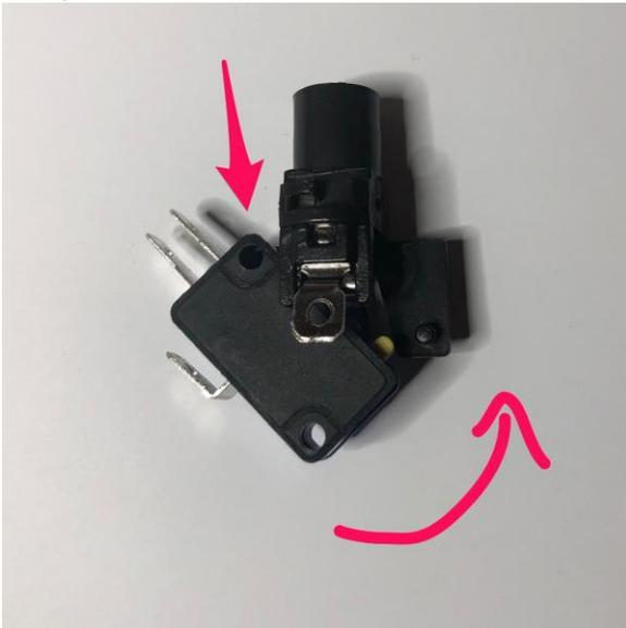
2. Push the quick connect receptacles onto the blades. The larger ones (0.250") attach to the LED blades, the smaller ones (0.187") attach to the switch blades. Note that COM is the blade on the bottom of the switch, and you can choose whether to attach the second one to either NO (normally open) or NC (normally closed).
